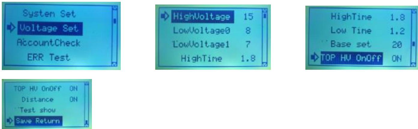
1. HighVoltage: set up the use of the strength of the value of the acquisition of large Mini range of machine 0-48. program scope: 0-24.
