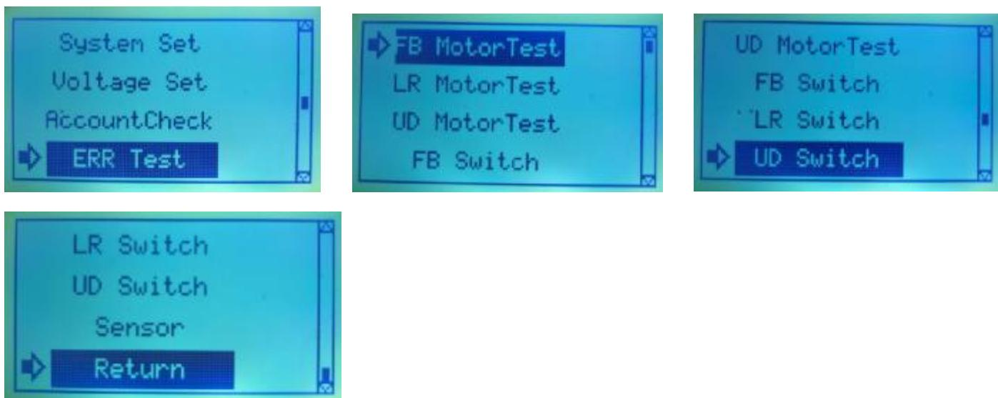
1. FB Motor Test: Before and after the test of the direction of the motor is running properly, the operation of the rocker around the front and rear to observe whether the operation, if the operation is normal before and after the motor, or motor failure or wire fault or motherboard failure. If the motor does not turn to observe whether the main engine working indicator light will operate with the rocker around the lights, if not bright for the motherboard failure, or motor or wire fault.
